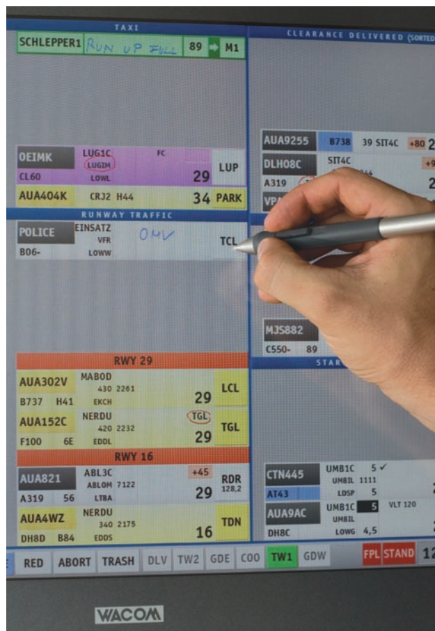
Figure 3: Digital Flight Strips System DIFLIS operated with pen input
