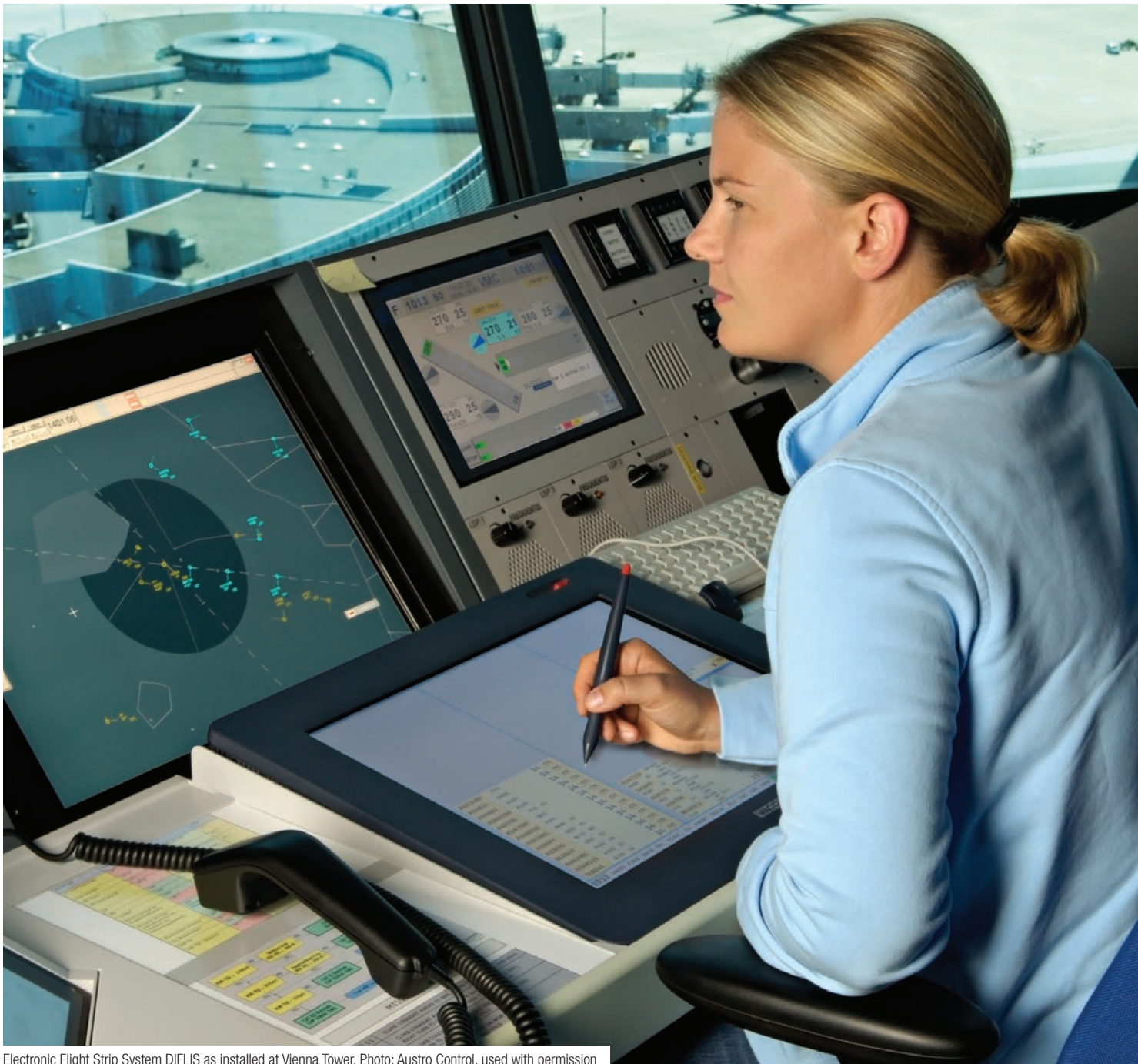
Electronic Flight Strip System DIFLIS as installed at Vienna Tower. Photo: Austro Control, used with permission
